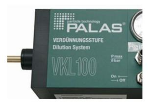
Depending on the model, the dilution steps can be configured for isothermal dilution of hot aerosols up to 200°C. Diluters made of stainless steel for operation up to 10 bar pressure are available and are used successfully worldwide for measuring chemically aggressive aerosols. The "partial flow dilution system" VDD is recommended for diluting large droplets (approx.  $> 5 \mu m$ ).
