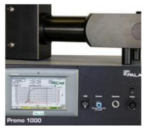
The success of the Palas® aerosol spectrometers is based on the development of a measurement method with white light source, 90° scattered-light detections and a measurement volume that was defined optically by the University of Karlsruhe, KIT.
